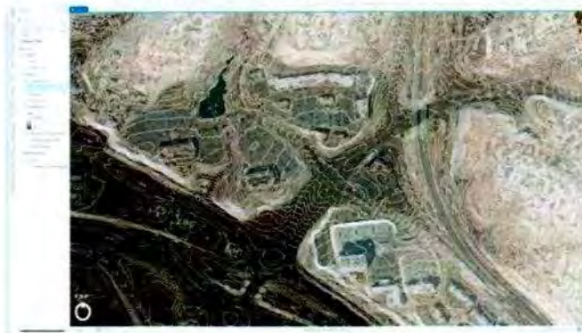
Figure 21 – One (1) foot contours derived from DEM data using Esri ArcGIS Pro
